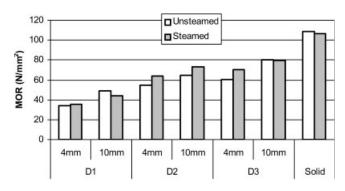
**Figure 3** Effect of handling of material (steamed– unsteamed) on MOR of finger-jointed beech wood (D1, D2, and D3 are durability classes of PVAc adhesive).
