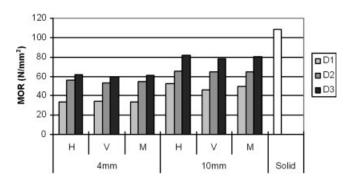
**Figure 2** Effect of PVAc adhesive class on MOR of unsteamed beech wood (H, horizontal; V, vertical; M, without orientation of fingers).
