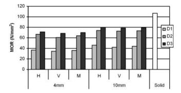
**Figure 4** Effect of PVAc adhesive class on MOR of steamed beech wood (H, horizontal; V, vertical; M, without orientation of fingers).
